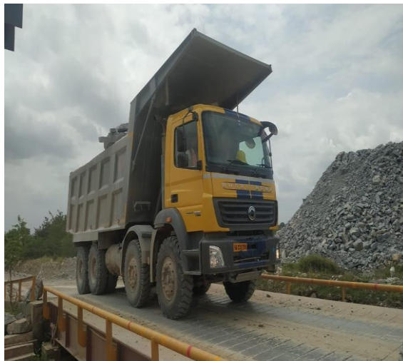
Vehicle entry to weigh bridge
